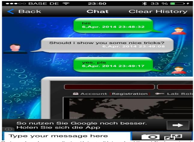
The image above shows an application-side input validation vulnerability and filter bypass issue in a bluetooth chat software of the apple mobile iOS. The attacker can send malicious messages to the victim via bluetooth protocol of the iOS device.
